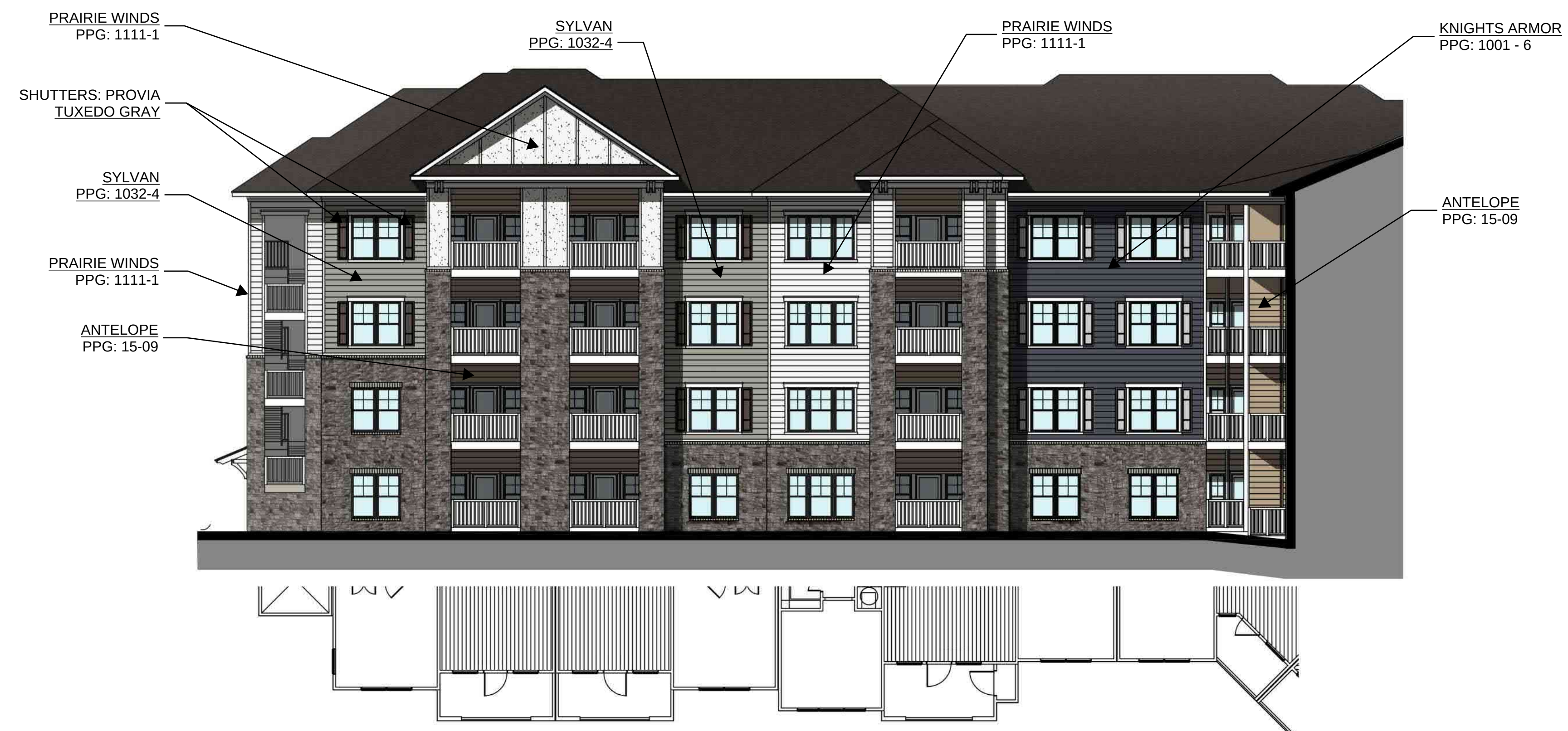
1 BUILDING TWO - EAST COURTYARD ELEVATION 3/32" = 1'-0"
