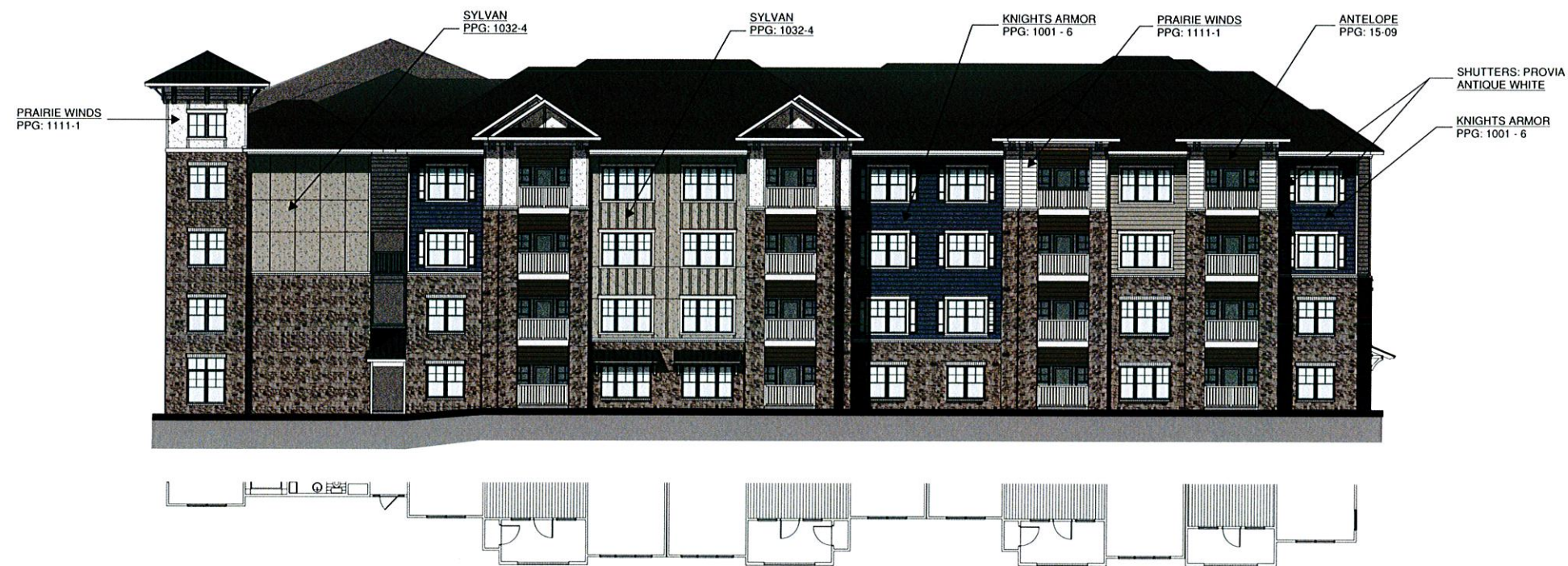
1 BUILDING TWO - EAST ELEVATION 3/32" = 1'-0"
