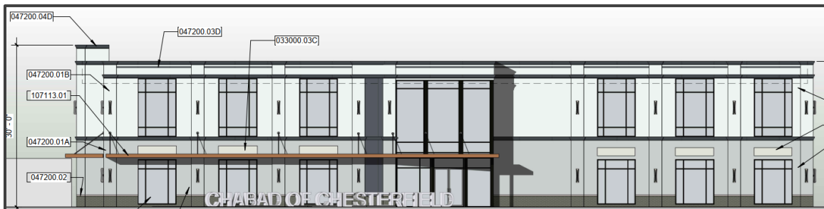
Figure 4: Proposed North side elevation facing Conway Road
