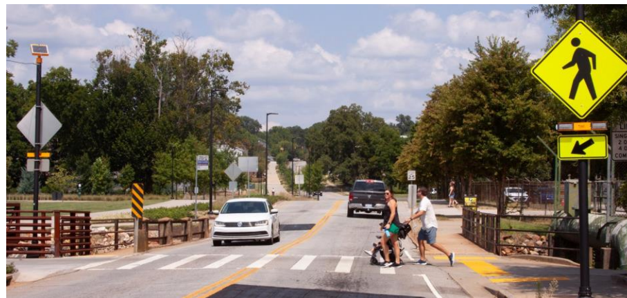
Rectangular Rapid Flashing Beacon (RRFB) have been shown to enhance pedestrian conspicuity and increase driver awareness at uncontrolled, marked crosswalks.
