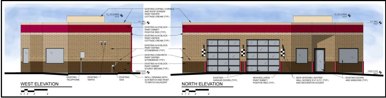
Figure 3: West and North Elevation
