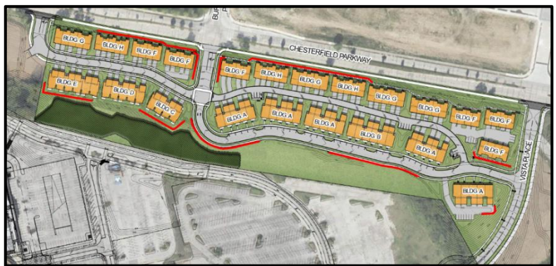
Figure 2: Proposed retaining walls within the development
