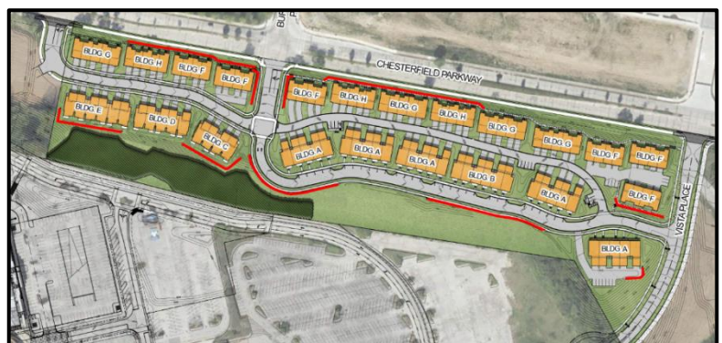
Figure 2: Proposed retaining walls within the development
