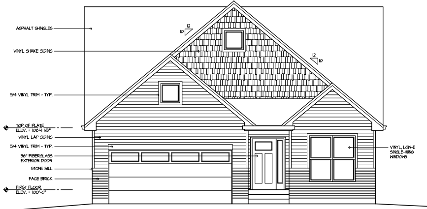
1 FRONT ELEVATION - TRADITIONAL 3-GABLE 1/4" = 1'-0"
