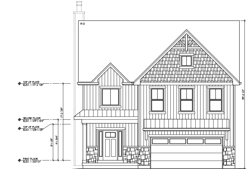
2 A4 FRONT ELEVATION - MODERN FARMHOUSE 1/4" = 1'-0"
