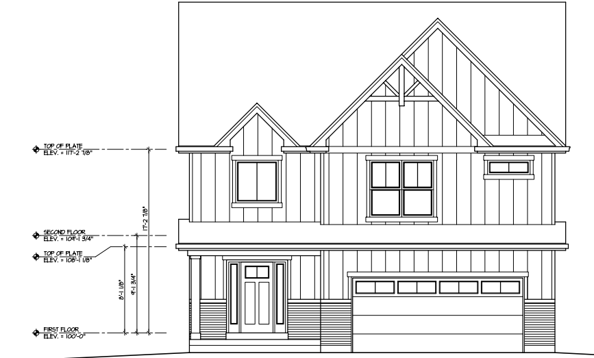
1 AS FRONT ELEVATION - MODERN FARMHOUSE 2 1/4" = 1'-0"
