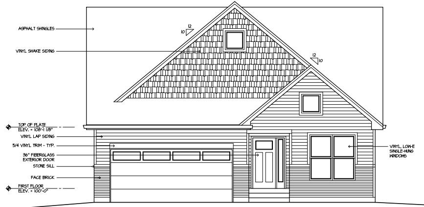
3 FRONT ELEVATION - TRADITIONAL 2-GABLE 1/4" = 1'-0"
