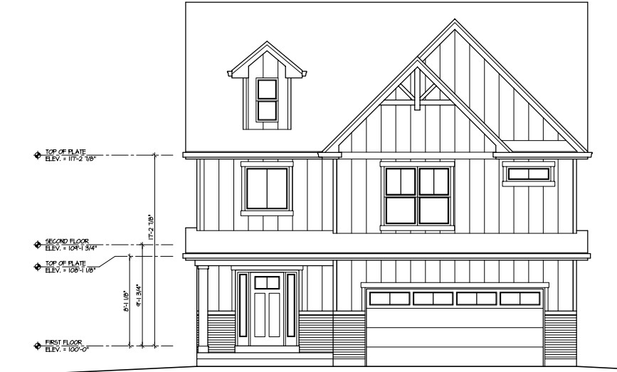
2 AS FRONT ELEVATION - MODERN FARMHOUSE 3 1/4" = 1'-0"
