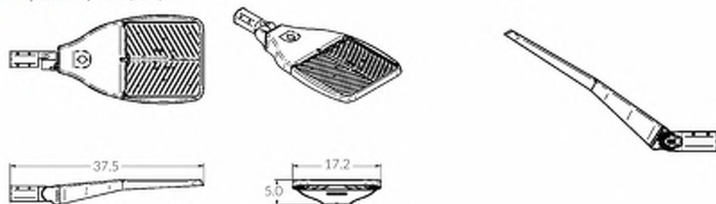
SAM Adjustable Slip Fitter (SLPF)
