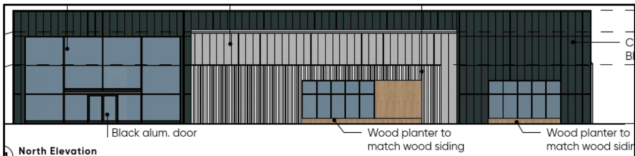
Figure 5: Front Elevation (North Side)
